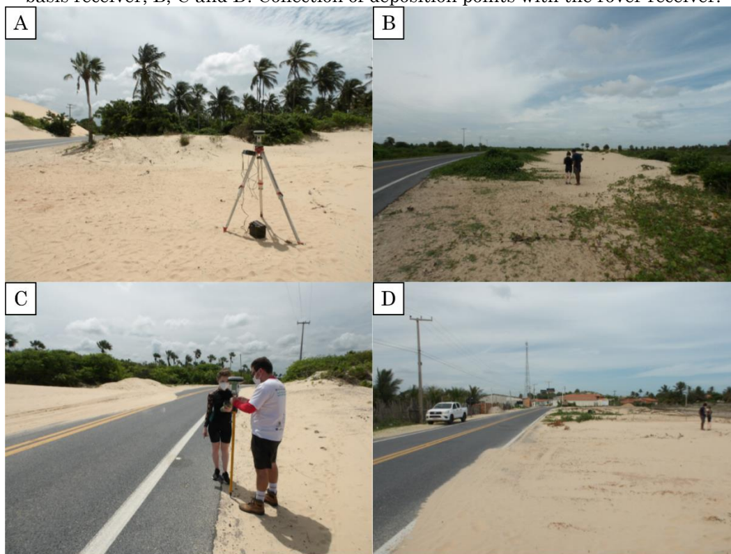
Figure 3 – Collecting control coordinates of sediment disposal area points. A. Geodetic GPS basis receiver; B, C and D. Collection of deposition points with the rover receiver.
