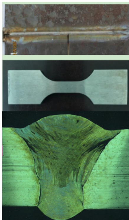
Figure 12. The welding sample with optimized welding parameters.
