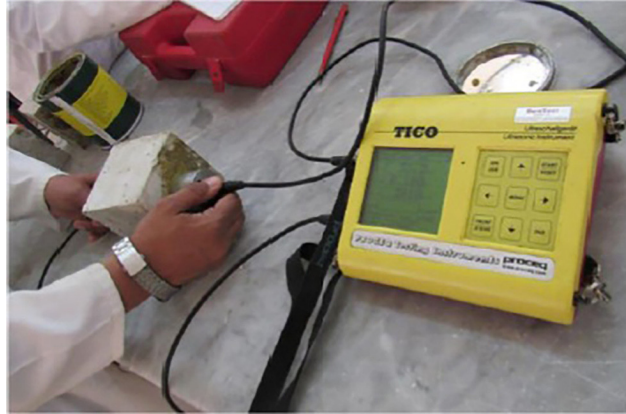
Figure 4: Ultrasonic testing device for evaluating wave velocity.
