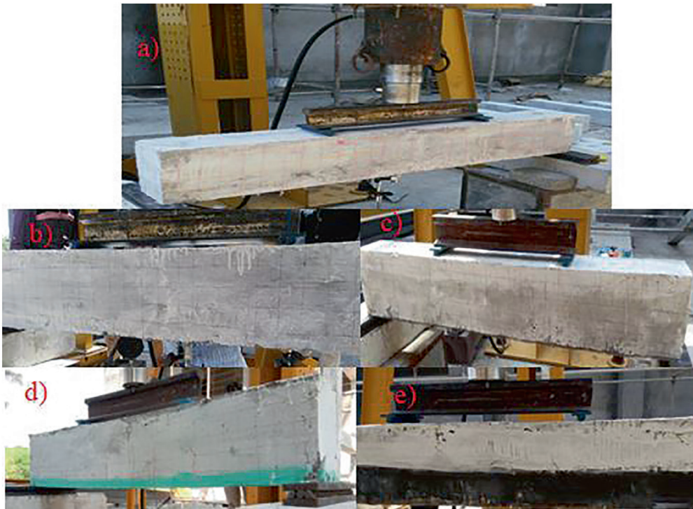
Figure 3: (a) Experimental test setup of beam specimen. (b) Failure pattern of control B0 beam specimen. (c) Failure pattern of PVCC layered BP3 beam specimen. (d) Failure pattern of basalt fiber fabric wrapped BB1 beam specimen. (e) basalt fiber fabric wrapped beam specimen.
