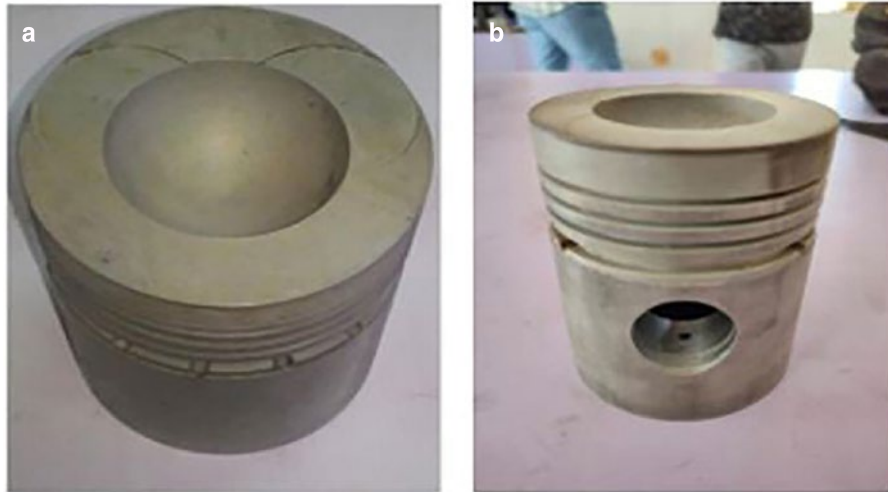
Figure 4: (a) Uncoated piston (b) plasma spray-coated piston.
