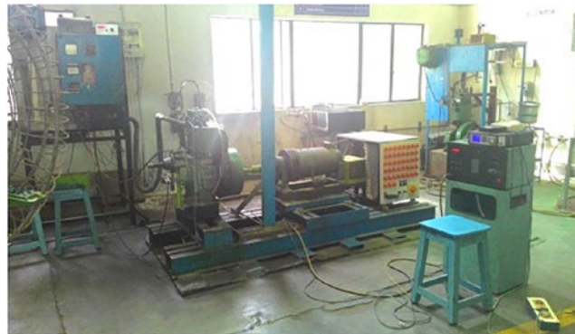
Figure 7: Photographic view of the engine test setup with instruments.
