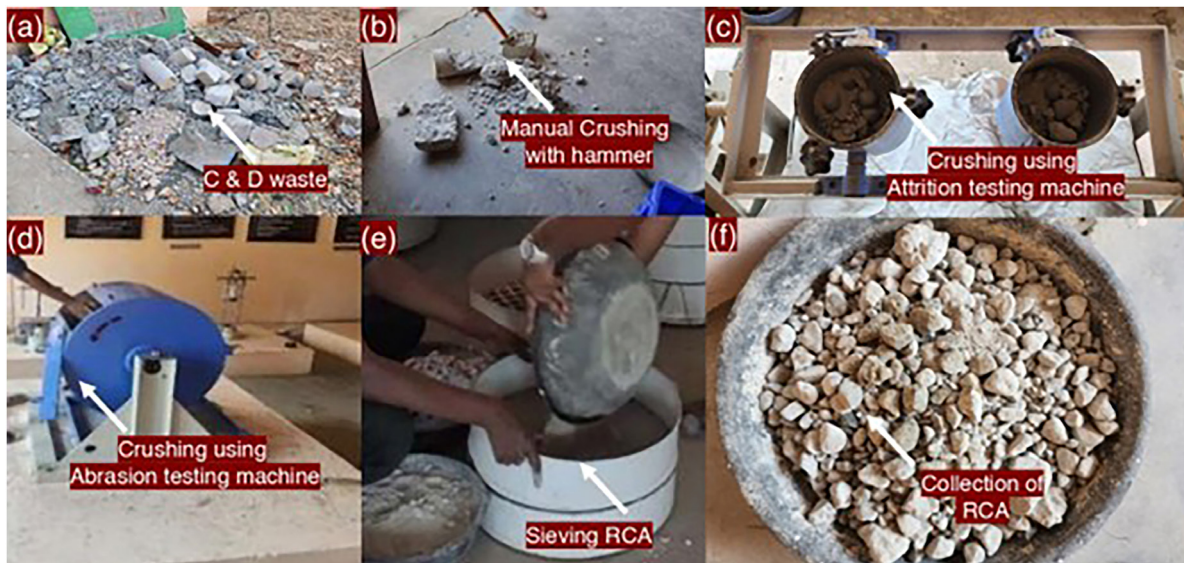
Figure 2: Preparation of RCA waste from renovation and demolition.
