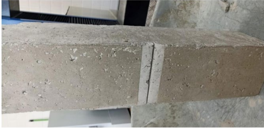
Figure 3: Example of a notch in a concrete beam submitted to the flexural strength test.
