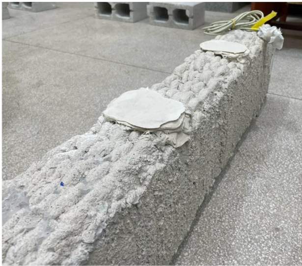
Figure 14. Regularization of the surfaces of printed beams.
