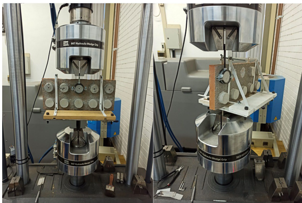
Figure 5. Shear adhesion strength testing apparatus.
