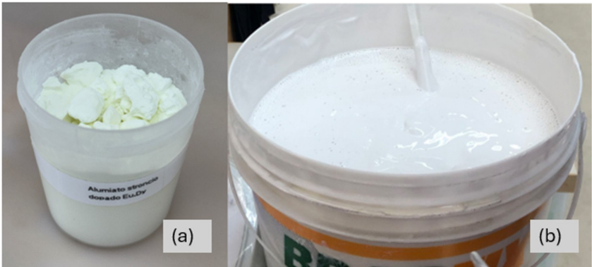
Figure 2. a) Phosphorescent compound – Strontium aluminate doped with Eu and Dy, b) Waterproofing membrane
