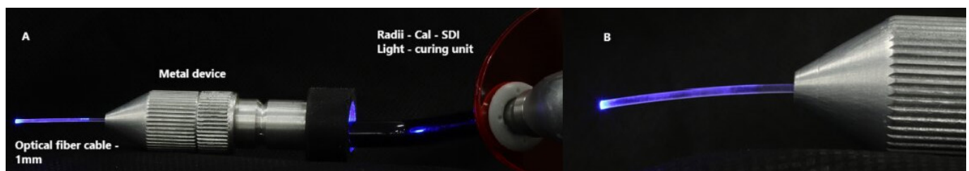
Figure 1. A) Complete fiber optic illuminating device being activated by a curing light. B) Fiber optic conducting the advised light from the curing light.
