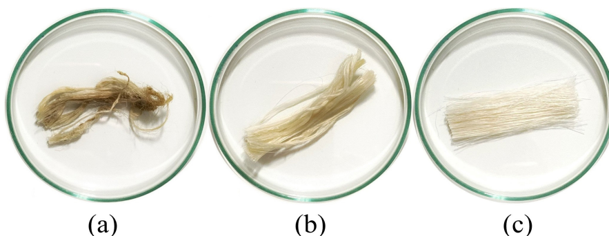
Figure 2. Curaua fiber samples: (a) Natural; (b) Washed; and (c) Washed and brushed.
