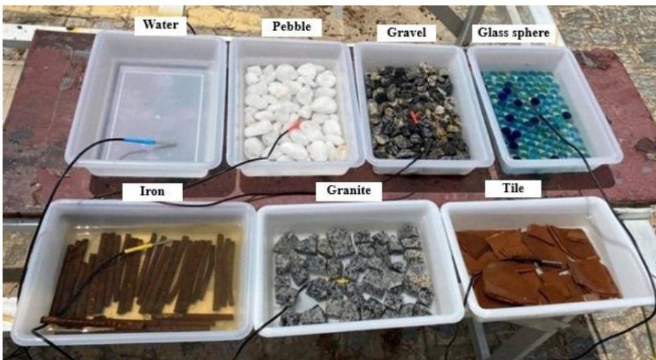
Figure 4. Temperature check of materials used. Prepared by the author, 2024.
