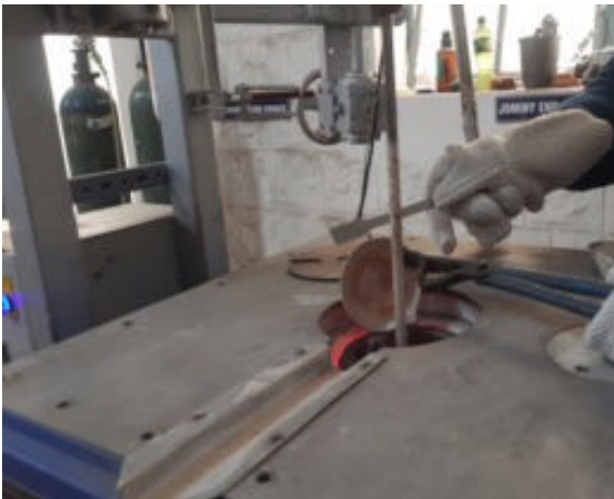
Figure 1. Stir casting set-up used in the investigation.
