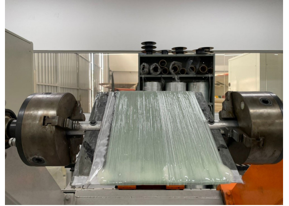
Figure 1. Composite manufacturing by filament winding process.
