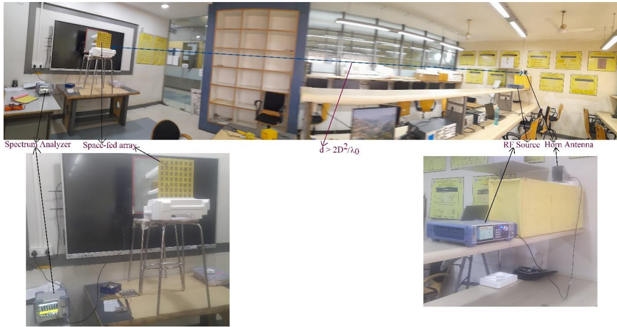
Fig. 7. Broadside gain measurement setup for 7 x 7 spaced fed array of E-shape MSAs
