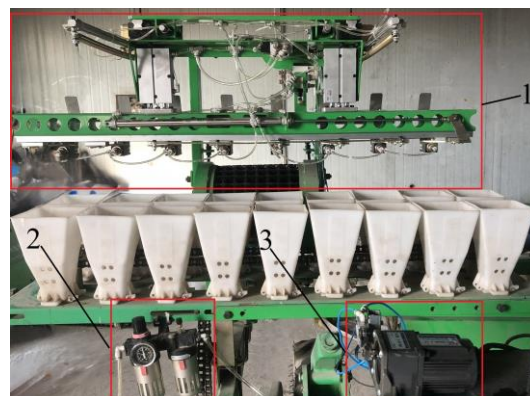
(1) Picking and supply mechanisms for seedlings; (2) pneumatic filter/regulator unit; (3) speed control motor
