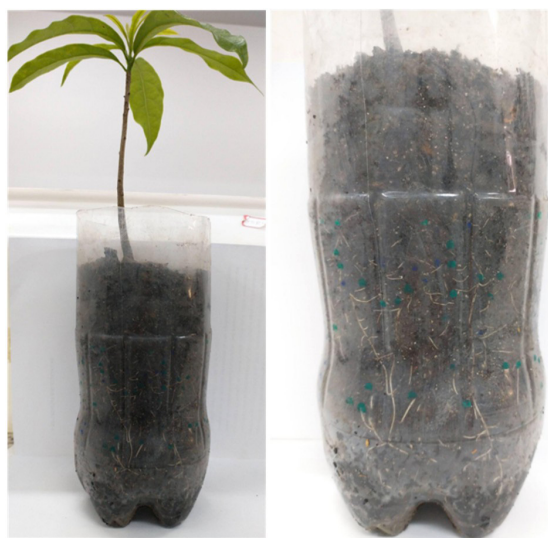
Figure 1. Rhizoboxes from PET bottles with vertical grooves for quadrant sampling.
