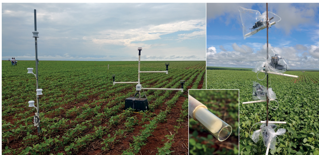
Figure 1 - Air samplers (right) and meteorological station to collect meteorological parameters (left) at different heights and detail of the PUF collectors (bottom box)
