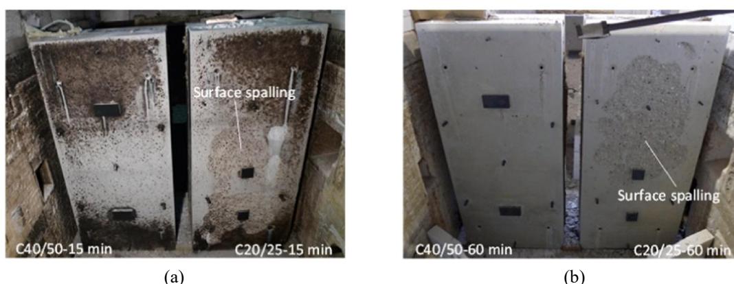
Figure 18 - Effects of fire on concrete prototypes after (a) 15 minutes and (b) 60 minutes of standard fire exposure
